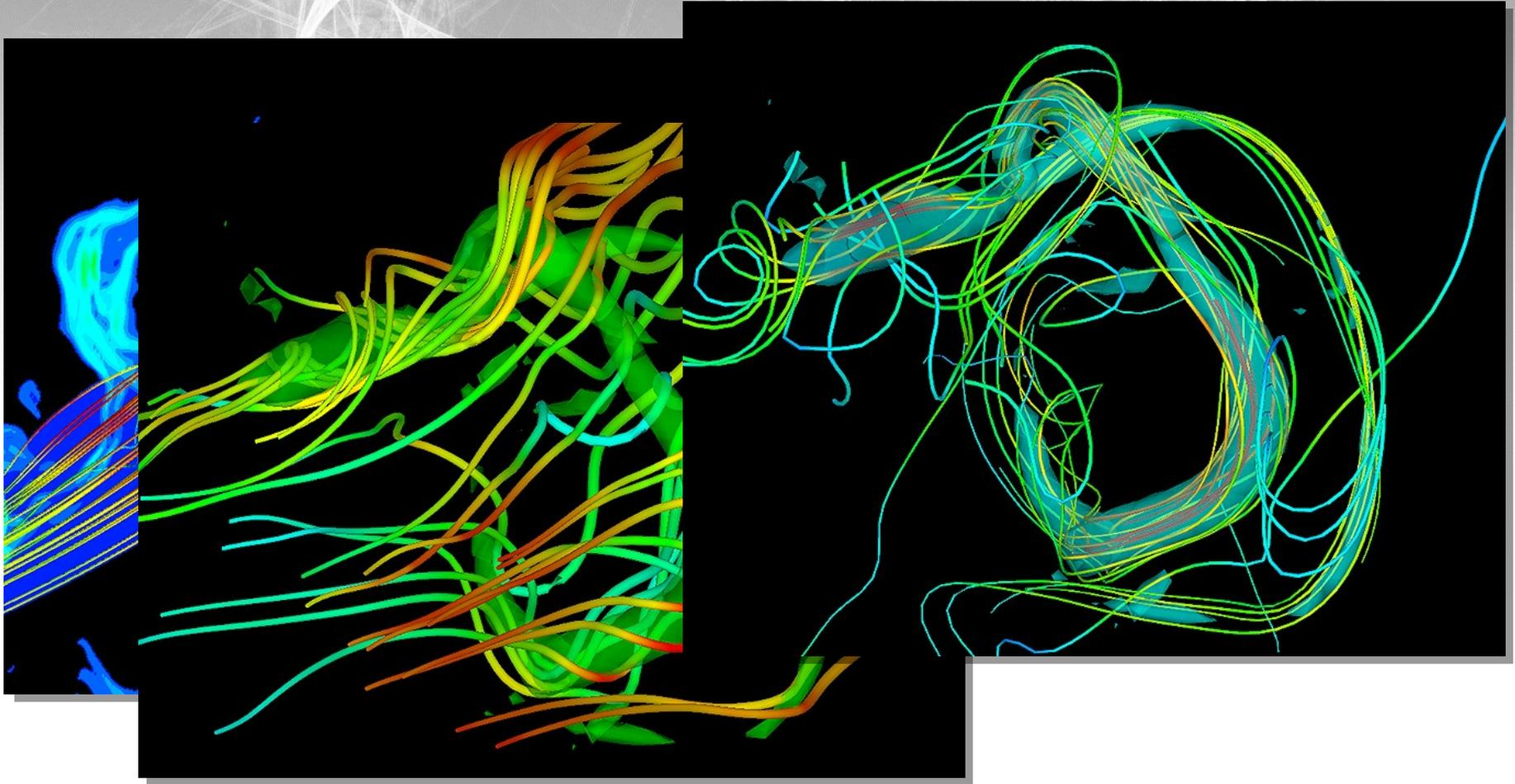
Q – criterion structure: the relationship of fluid stream lines and vortex filaments inside and outside Q - isosurface.
